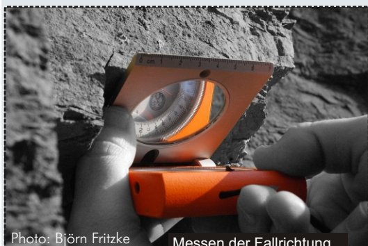
Messen der Fallrichtung Measuring of dip direction
